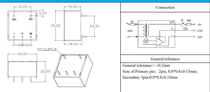
Instruction for use of the voltage sensor model CHV10A15D25-T:
